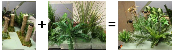
Fig. 5: (Left) Trunk-only environment for training the HMM model for Trunk category; (Middle) Leaf-only environment for training the HMM model for Leaf category; (Right) Combined environment for testing.
