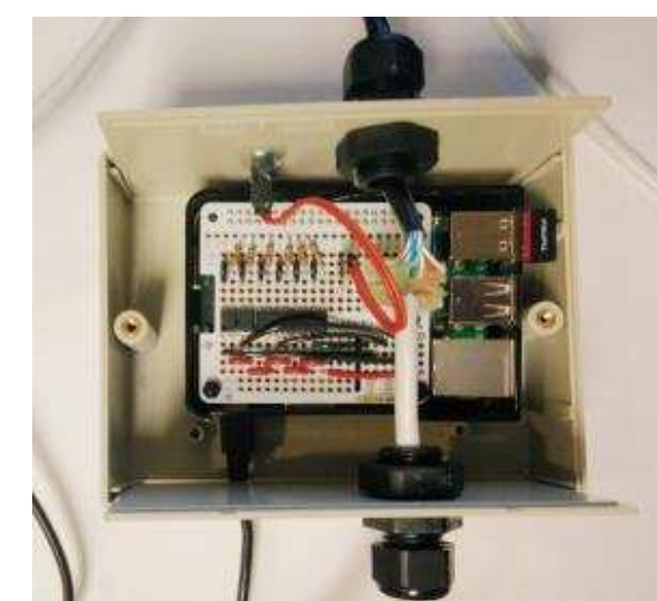
Autobed computer and circuit
